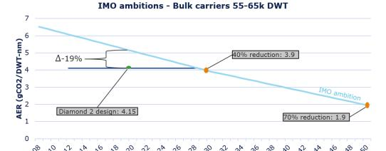
The estimation was done by using a large set of AER data for the 25% best performing Crown 63 vessels (the reference design of Diamond 2) currently in operation, as reported to EU MRV, and further by applying the theoretical percentage difference in fuel oil consumption as weighted over the expected operational profile. The estimation is believed to be conservative.
